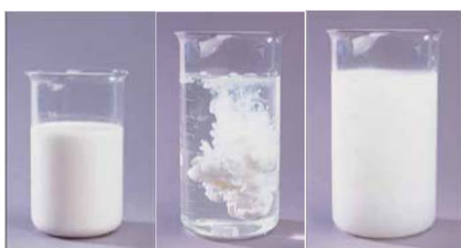
Fig. 3: Mixing of suspension concentrate in water results a stable suspension (Photo Courtesy: Bayer Crop Science)
