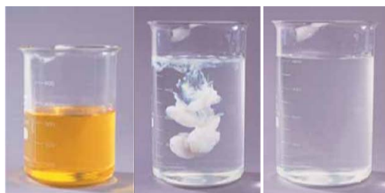
Fig. 2: Mixing of soluble liquid in water results a clear solution (Photo Courtesy: Bayer Crop Science)
