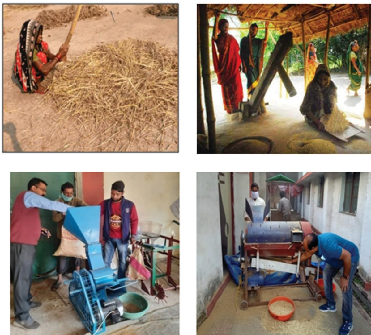
Fig. 1: Available methods of threshing and pearling of finger millet:(a) manual beating with stick, (b) Pearling with dhenki ,(c) Vivek finger millet thresher cum pearler, (d) IGKV finger millet thresher cum pearler
